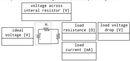
**6.** Using the voltage across the internal resistor and the current flowing around the circuit, you can now use *Ohm's law* to calculate the internal resistance, R<sub>i</sub>, of the power supply you are using. Perform this calculation, showing the initial formula and all steps for the calculation in the box below.
