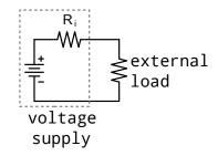
When there is no load on the voltage supply, no current flows through the internal resistor, so the voltage drop across the internal resistor is zero. You can verify this with *Ohm's law*:
